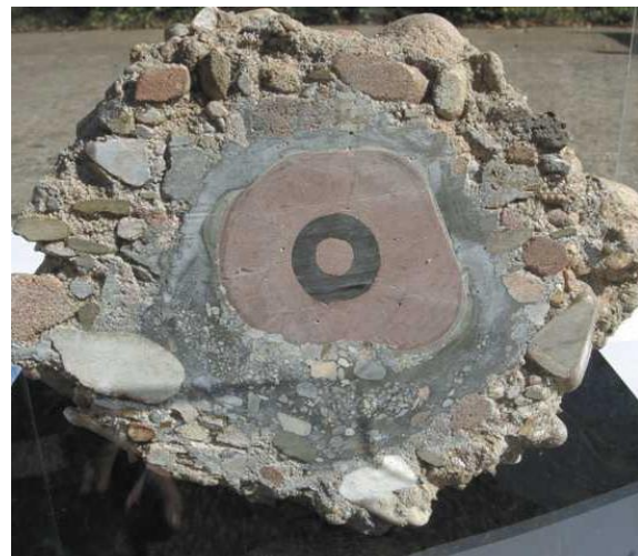
Figure 4 Mechanical interlock grout body/soil
